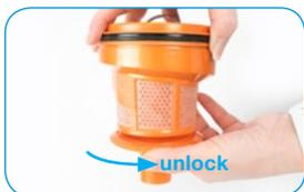
5. To separate the mesh filter from the filter cone, turn the base of the mesh filter to the “unlock” position and gently remove. The filter cone and mesh filter can be washed using lukewarm water. The filters need to be air dried for 24 hours before it can be reinstalled into the machine.
